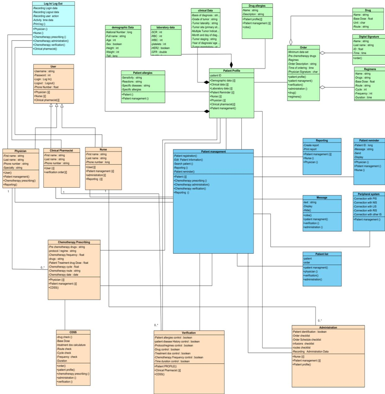
Appendix 2. A. The class diagram of the guideline-based workflow software system
